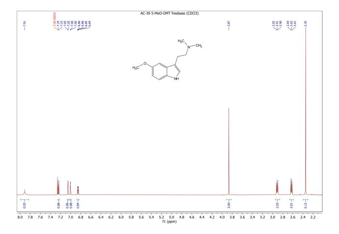
Lab Notes:The sample contained the expected compound 5-MeO-DMT in itsfreebase form without any detectable impurities.
