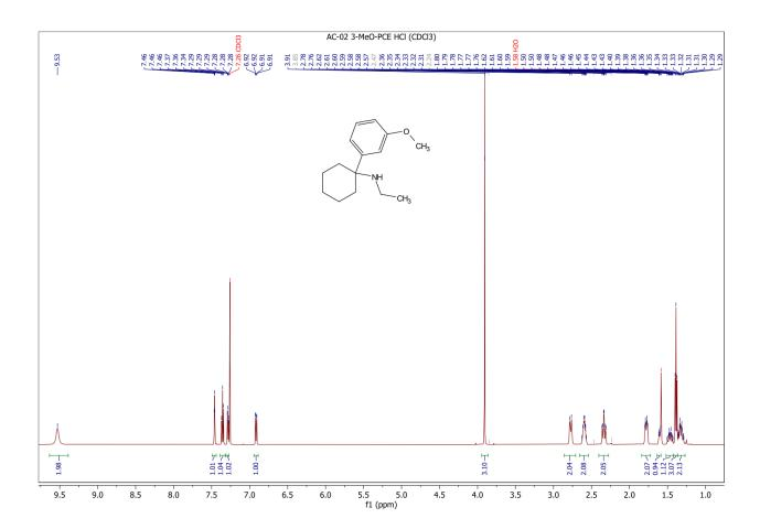
**Lab Notes:** The sample contained the highly pure compound 3-MeO-PCE in its HCl salt form with barely any <sup>1</sup>H NMR active impurities.
